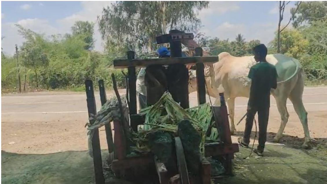
Figure 3: Treaded wooden crushers rotated by the animal
